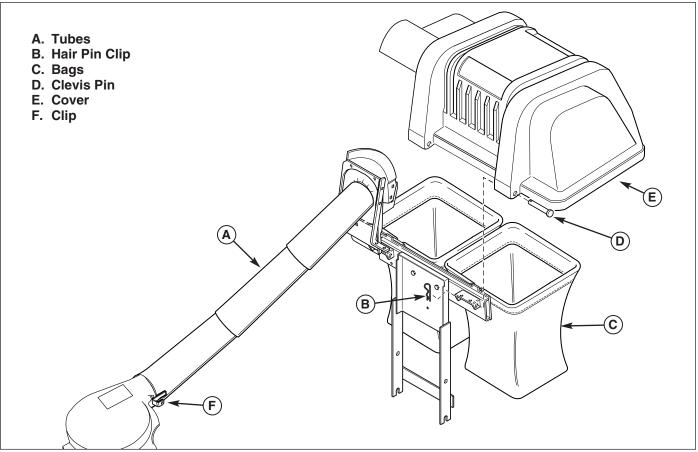
Figure 9. Normal Removal & Installation
